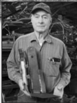
Paul showing one of the knives he makes. It runs about 7 or 8 inches deep, lifts and loosens the soil and spreads the nitrogen out behind the wings.
